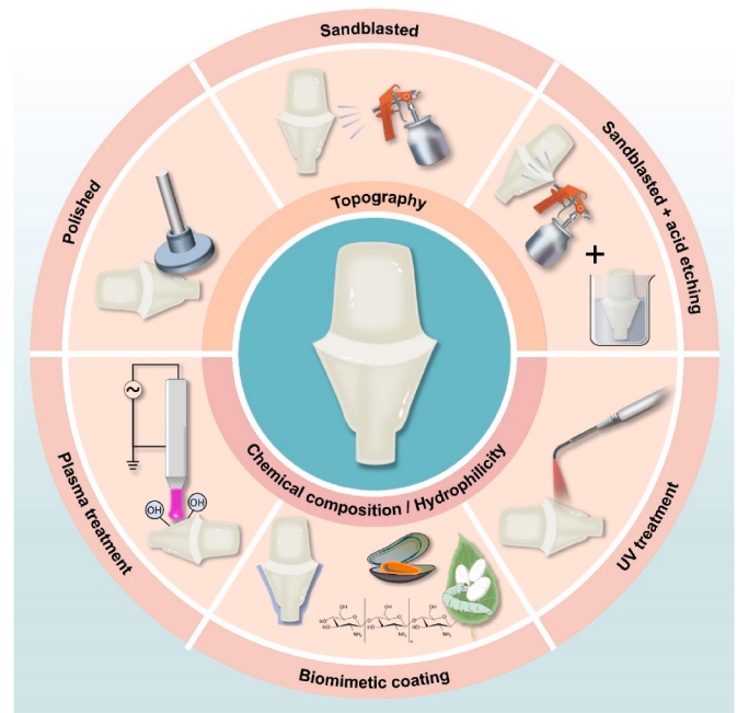
Fig. 1. Surface modification of zirconia abutment.
